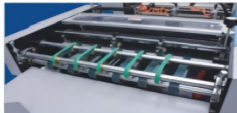
瓦楞曲纸系统 Corrugated Delivery A corrugated delivery system collects papaer easily
